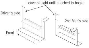
resin. Keep the steps parallel to the side frame and attach the rear mounting to the top of the side frame photo: Bogie step and speedo drive.jpg, but note the front mounting leg has yet to be bent down to meet the bogie frame in the photograph.
