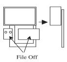
49.7) Cut the pipe extensions off the exhaust silencers C9 as shown right.
