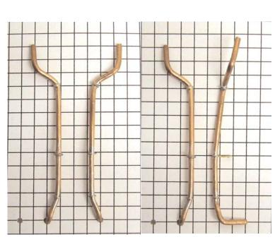
The 122 stacks do not have the top bends as shown here (left), but simply go straight up either side of the small destination box. Above the gutter they curve gently back and then turn back vertical as shown right (not to scale). Originally the exhausts turned inward above the destination box and joined in a central collector box. This box scales to approx. 7mm x 7mm x 3mm. The overall height of the stacks is the same as the 121 stacks in the illustrations (left).
